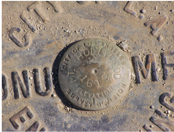
Figure 121: Mt. Hollywood peak: City Of Los Angeles Engineering Monument Marker. View S. Photo: ICF Jones & Stokes, August 2007.
